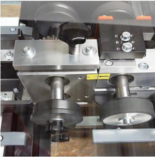
Tool-free changing station for/for clip relief use
