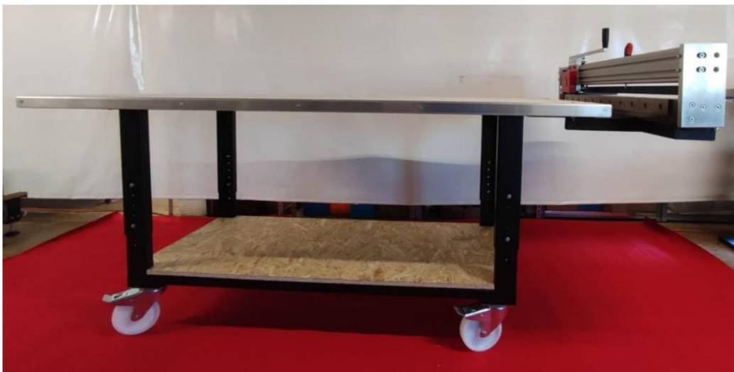
Cutting and cross-cutting table (optionally including hand scissors TS 1000 or TS1250 mm)
