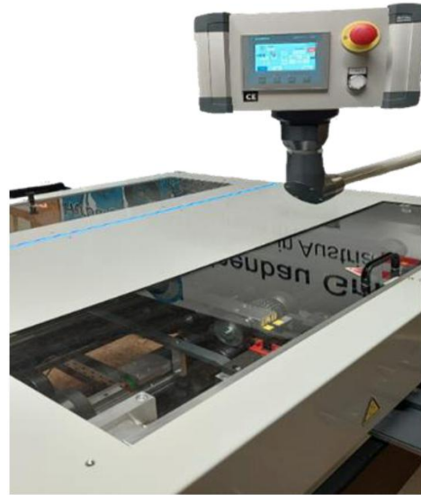
Pivoting control arm for all-round Movement and state-of-the-art touchscreen display – Made by Siemens
