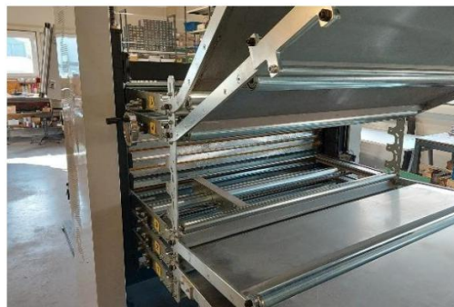
Infeed to material feed lift
