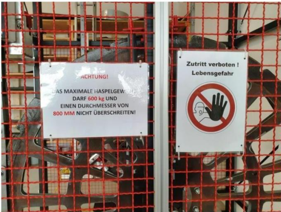
Protective grille on the coil tower
