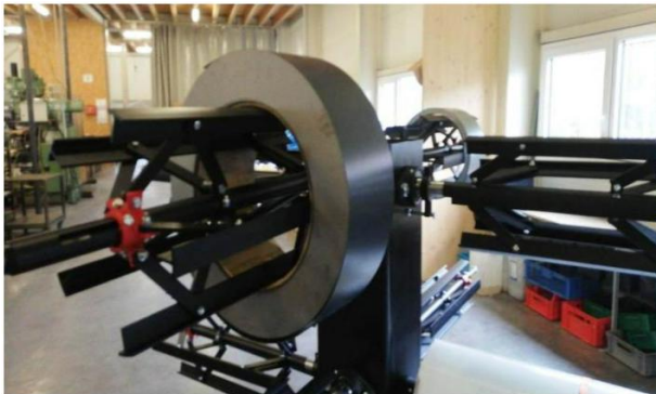
Station with sheet metal coil
